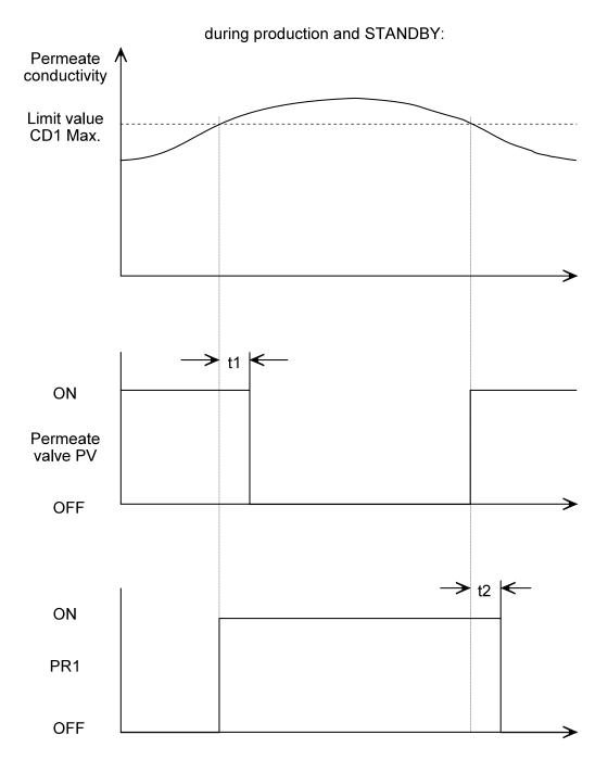
Delays: t1 and t2 are permanently set to 10 seconds
